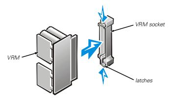
Figure 8-14. Installing the VRM
